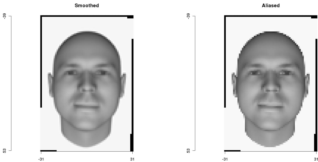
Figure 2.8: An important example of image resampling: a face image is rotated, translated, and scaled so that the (centers of) the eyes of the subject are located at predefined positions. The two images illustrate the difference resulting from proper frequency conditioning via smoothing (left) and the direct use of the affine transform of Equation _{TM:2.76}
